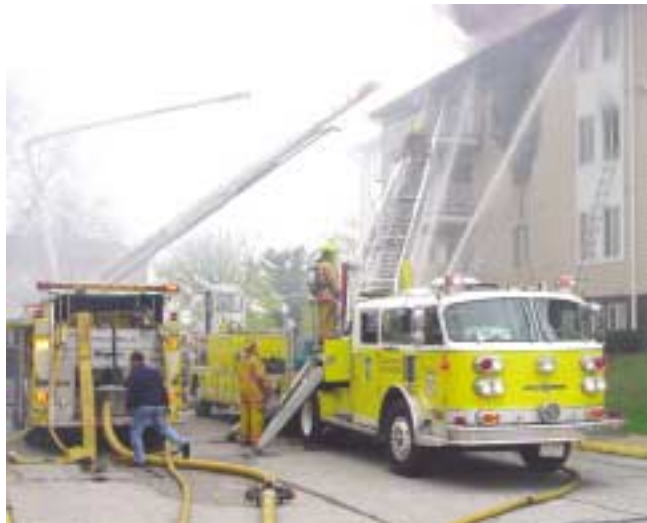
(Fig. 2.1) Good aerial apparatus access at an apartment fire. This fire lane is wide enough to allow passing even when aerial outriggers are extended, and it is located a proper distance from the building to facilitate aerial operations.
