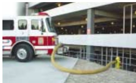
(Fig. 2.15) Here is a pumper connected to a hydrant by its front-mounted suction hose. The pumper end of the hose has a swivel to facilitate reaching hydrants on either side.
