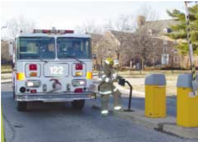
(Fig. 2.9) The delays caused by electronic gates can be minimized by providing the fire department with access cards or remote access controls.
