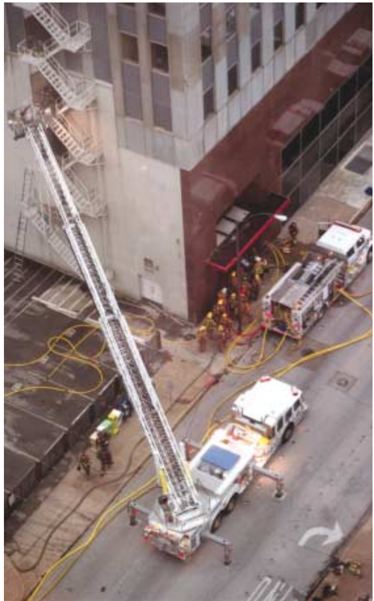
(Fig. 1.2) A view from above of both a pumper (top) and an aerial apparatus (bottom), in this case a platform type of aerial.
